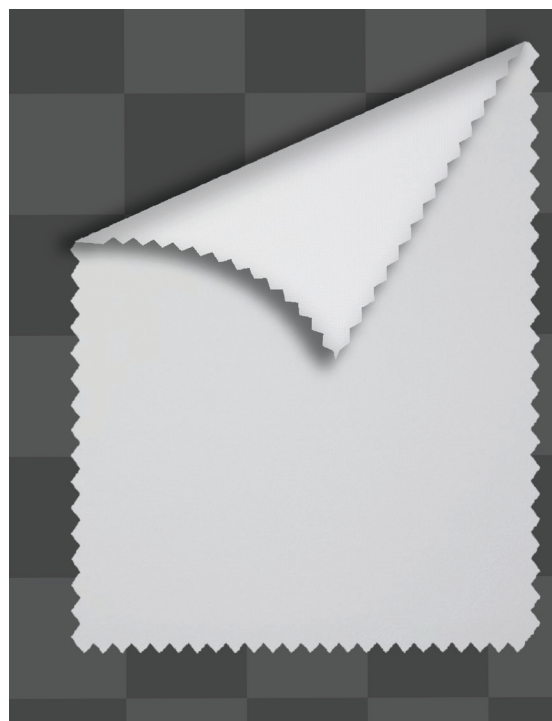
NFPA-701 flame Retardant certified. Recommended transfer settings for sublimation are 374°F-410°F for 40-100 seconds at 40psi.
